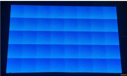
After you assemble the whole LED screen, you need to send a .CON file, in order to make the whole LED screen show image in one piece. You will get the perfect image below after sending a .CON file to the above LED screen.
