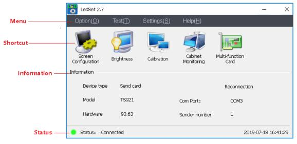
**Note**: You have to connect the USB cable from PC to sending card **before** you do the setup (such as generating .RCG&.CON file, brightness control and monitor and etc.).
